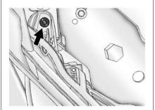
2. Remove the screw from the headlamp assembly.
